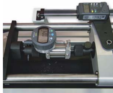
OPTIONAL EXTENSOMETER (SM1002A) FITTED TO TL SPECIMEN
